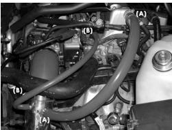
Take the 18" 15.9mm hose and press one end over the crank case port and the other end over the 3/4" port on the intake(A). The 20" 4mm hose has been connected to both ports (B).
