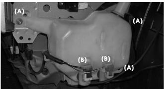
Remove the three m6 bolts holding the reservoir tank in place (A). Remove the 2 pin connector pins from the two washer motors (B). Remove the stock reservoir bottle from the car frame.
