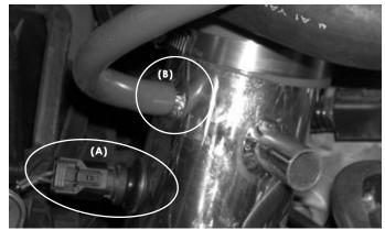
Take the air temperature sensor and press it into the grommet installed earlier (A). Take the 20" 4mm hose can press one end into the brake booster port and press the other end over the 3/8" port on the intake (B).
