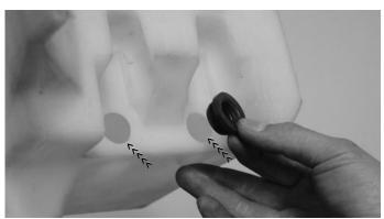
Remove the stock motor grommets from the stock reservoir tank. Press the two stock grommets into the pre-drilled 21mm holes in the new reservoir bottles.
