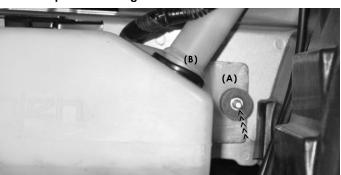
Align the three holes in the reservoir tank to the three pre-tapped holes located in the car frame. Screw the long stud on the vibra-mount over the reservoir tank and into the pre-tapped hole until the tank is firmly fastened(A). Firmly press the end of the spout into the grommet until a proper seal has been achieved(B).
