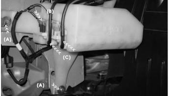
Use the m6 x m25 bolts and fender washers to secure the two extended legs on the reservoir tank (A).
