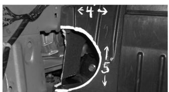
Once the tank has been removed cut a  $4" \times 5"$  open on both sides of the splash guard. This will allow access to the bumper area for the filter.
