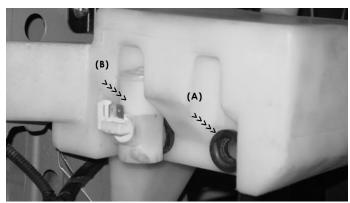
Once the stock grommets have been pressed into the pre-drilled holes(A) take the stock motors and press them into the stock grommets(B).
